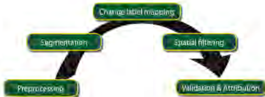
Figure 1. The typical arc of the LandTrendr workflow. During preprocessing, annual (or super-annual) Landsat images from approximately 1985 to present are acquired, normalized, and masked for clouds. In the segmentation phase, algorithms simplify the noisy time series of imagery into time periods in every pixel’s “life history” when vegetation cover is either increasing, decreasing, or remaining stable. These time periods are then expressed in map form during change label mapping, allowing description of landscapes by the different processes of interest: slow mortality, abrupt mortality, growth, or sequences thereof. Pixels in these maps are grouped into patches and isolated pixels removed during the spatial filtering phase, leading to final maps that can be expressed as either raster or vector (patch) attributes. Finally, these maps must be compared against other reference data to determine their robustness.
