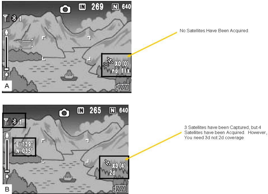
Figure 4. The display of the Ricoh camera showing (A) no satellite coverage and (B) 2d satellite coverage.
