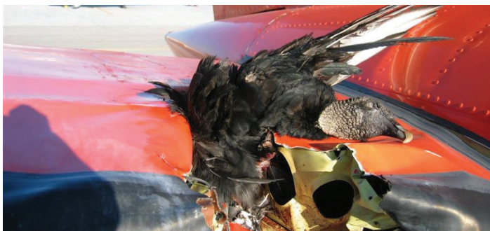
T-44 aircraft from VT-31 Training Air Wing Four, that struck a Black Vulture. Source: VT-31 Safety
